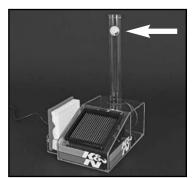
4. Place the K&N High-Flow Air Filter™ in the front opening. Watch the ball rise, demonstrating the increase in airflow with the K&N High-Flow Air Filter™.
