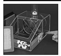
1. Put the toggle switch located on the right hand side in the up or on position.
