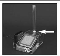
3. Place the supplied typical paper air filter in the front opening. Watch the ball drop because the air restriction is too great to elevate the ball in the tube.
