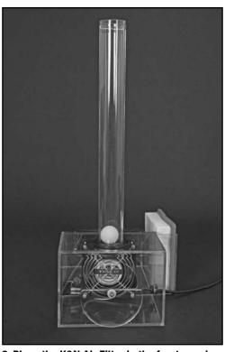
2. Place the K&N Air Filter in the front opening, the ball may drop to the bottom of the tube.
